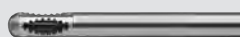
26208 SA Shaver Blade GYN , straight, sterilizable, concave cutting edge, double serrated, oval cutting window, diameter 4 mm, length 32 cm, for use with DRILLCUT-X® II Handpiece 26 7020 50, color code: blue-green
