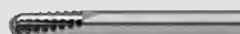
26208 SB Shaver Blade GYN , straight, sterilizable, double serrated cutting edge, rectangular cutting window, diameter 4 mm, length 32 cm, for use with DRILLCUT-X® II Handpiece 26 7020 50, color code: blue-yellow
