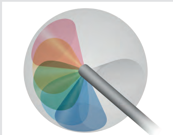
ENDOCAMELEON® with variable direction of view, isometric view
